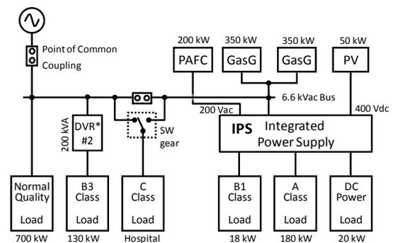
Figure 1 System Configuration of the Sendai Microgrid
