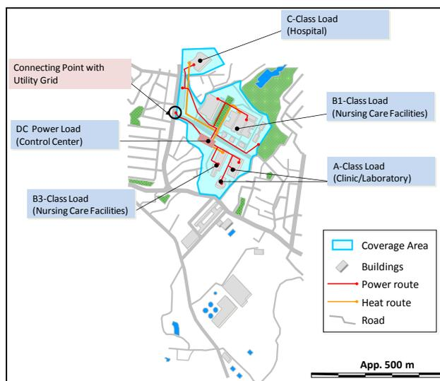
Figure 4 Supply Area of the Sendai Microgrid
